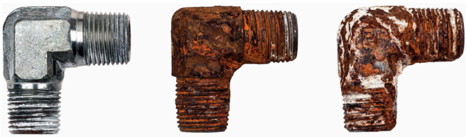
Corrosion of current carbon steel adapters after 650 hours of exposure to salt spray testing.
